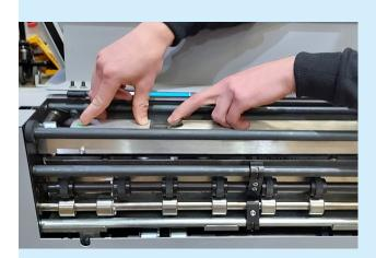
EasyBlade quick release mechanism.
