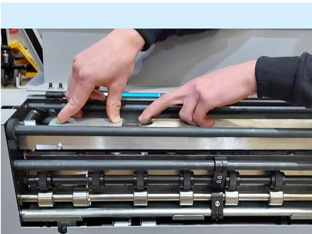
*EasyBlade quick release mechanism.*
