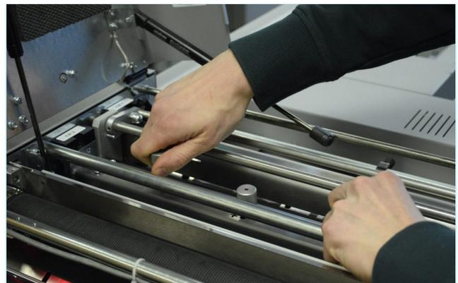
*The Easyblade quick release mechanism enables changing crease blade for different jobs, without any special tools in less than 30 seconds. Extremely useful when changing between a perforation job and a creasing job.*
